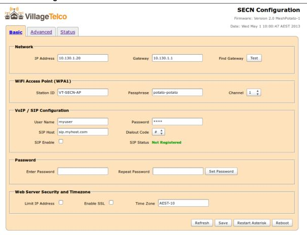
The Basic SECN Configuration screen may be accessed by pointing your web browser to the IP address of the MP device. A newly flashed device will not have a root password set and thus the web interface will not require authentication.
