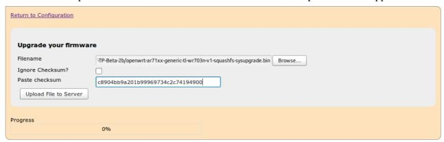
If the checksum comparison is correct, you may select whether to preserve the current device configuration (eg IP address, SSIDs, passwords etc), then select *Upgrade Firmware* to begin the flash process.
