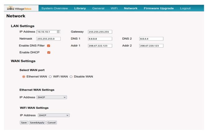
The Network screen allows you to set up the networking parameters of the Digital Library. Select *Network / Network from the top menu*
