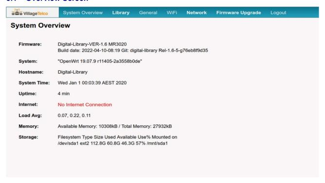
The System Overview screen displays the device identification and software version data, along with some operational information including time, Internet connection status, system load, system memory utilisation, and storage usage.
