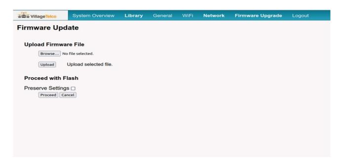
This screen allows you to update the firmware on the device by uploading a sysupgrade file from your PC.
