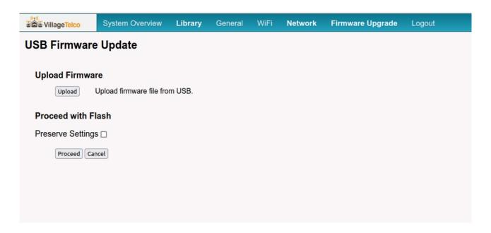
This screen allows you to update the firmware on the device by uploading a sysupgrade file from a USB memory stick installed on the Digital Library device in lieu of the memory device containing the normal library content.
