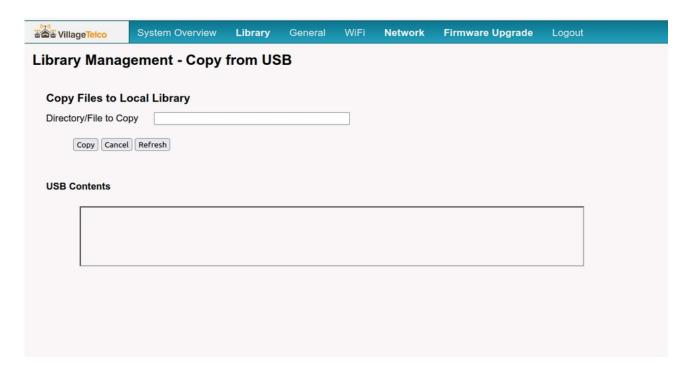
The *Library Copy* screen allows you to copy files or directories from a Secondary memory storage device onto the main Library storage device.
