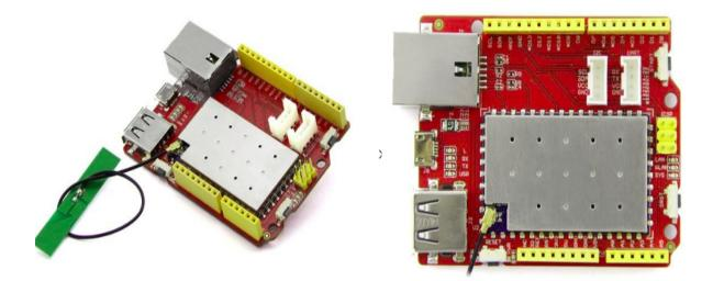
This device is based on the Atheros AR9331, @400MHz chipset.
