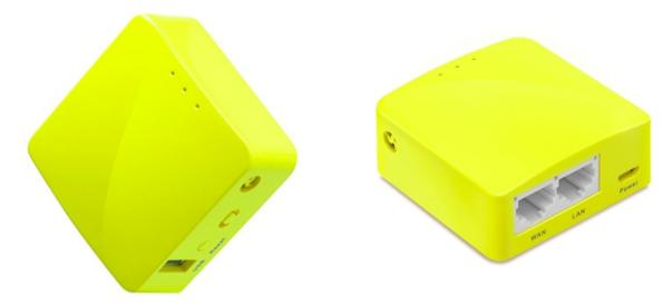
This device is based on the MediaTek MT7628NN @580Mhz chipset.
