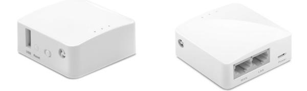
This device is based on the Atheros AR9331, @400MHz chipset.
