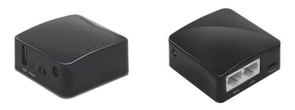
This device is based on the Atheros QCA9531, @650MHz chipset.
