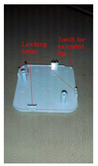
Note the location of the three "tangs" that engage the teeth in the inside edges of the enclosure base. Note also the single tooth that engages the extended lip in the enclosure base (just to the right of, and above, the reset hole in the front of the unit).
