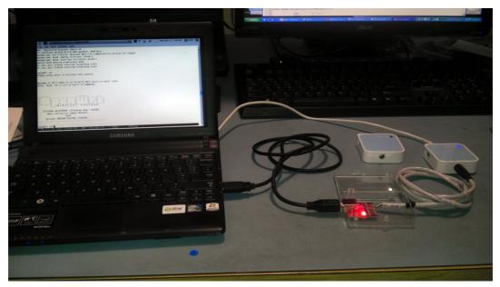
After "bricking" both of my TL-WR703N routers by flashing with "bleeding edge" (r29140 at that time and fail-safe broken), I decided to buy some sort of serial TTL level-shifter so that I could access U-Boot and the OpenWRT console.
