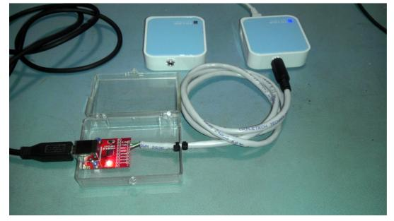
When the CP2103 adapter arrived in the mail, it only took a few minutes to solder it to the appropriate holes at the end of the adapter board. Since I knew that the solid green wire in my cable was ultimately connected to TP\_IN, I soldered that to the board's TXO, the white/green wire to RXI and my ground wire to GND.
