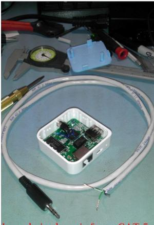
I used single pair from CAT-5 cable for TP\_IN, TP\_OUT and a single wire from a second pair for TP\_GND.
